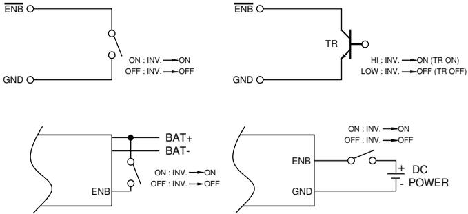
Note : At one time, only one remote function should be used to control the inverter. The maximum voltage value is 60VDC.
