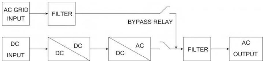
The inverter features IGBT technology which, minimizes weight and dimension, while enhancing output short circuit reliability and overload capacity.
